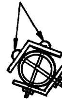
Figure 13-7. Suggested Repair for Control Rods or Tubes
